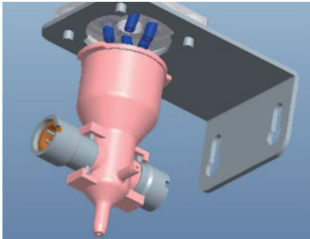
Improved DC impedance technology is used to count and size the RBC and PLT. The smaller counting aperture (50  $\mu\text{m}$  in diameter) provides better performance on samples with low PLT.
