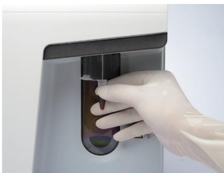
Running capillary blood through the sample probe directly is more convenient for the users in children's hospitals, etc. For Prediluted mode, BC-5000 has higher dilution ratio than other 5-part hematology analyzers, thus it brings a better mixing effect.
