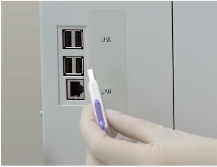
4 USB ports are located on the instrument's left side. They permit BC-5000 users to transmit data conveniently and connect with printers, keyboard, mouse, barcode scanner, etc.
