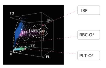
With the SF Cube cell analysis technology, Reticulocytes are differentiated from the other red cells by their reaction with fluorescent stain. Besides the traditional parameters such as RET# and RET%, BC-6800Plus provides data concerning immature reticulocytes (IRF), which can assist in early diagnosis of anemia and monitoring the bone marrow response to therapy.
