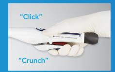
Handle must be fully squeezed until it comes in contact with instrument body.
