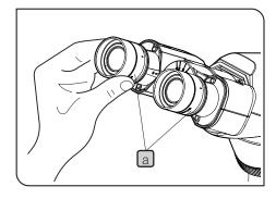
The diopter adjustment is to compensate for the difference of eyesights between left and right eyes of the observer.
