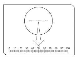
When the eyepiece is equipped with the eyepiece micrometer
