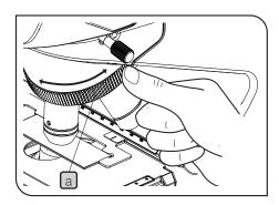
Hold and rotate the revolving nosepiece a so that the objective to be used comes exactly above the specimen (specimen slide).
