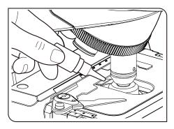
O The designated immersion oil should be applied to the top lens of the 100X oil immersion objective. Otherwise, the observed image will be unable to be focused on.
