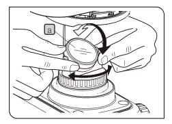
This is a reflection mirror to be used for microscopic observation using natural light in place of the LED illumination in a location where power supply is not available.
