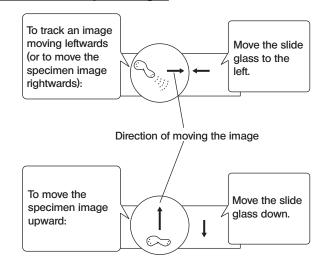
The image observed through the microscope moves in directions opposite to the actual up-down and left-right movements of the specimen.
