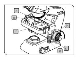
CAUTION If the specimen holding lever c is returned with a strong force or the knob a of the specimen holding lever c is released in the middle, the slide glass may break.
