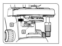
4. When cleaning the condenser, move the lever a to the left end, lower the condenser with the condenser up/down knob b, and remove the condenser. Then, clean the upper lens area. When attaching the condenser, engage the condenser to the condenser attaching part and push the engaged part upward until it touches the top.
